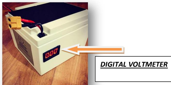
FIGURE-4 LITHIUM ION BATTERY VOLTMETER
